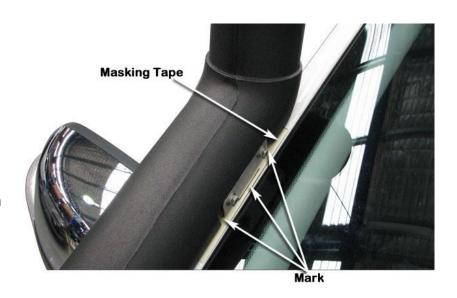
Remove the snorkel body (Item 1) from the vehicle and remove the upper mounting bracket (Item 3) from the snorkel body.
